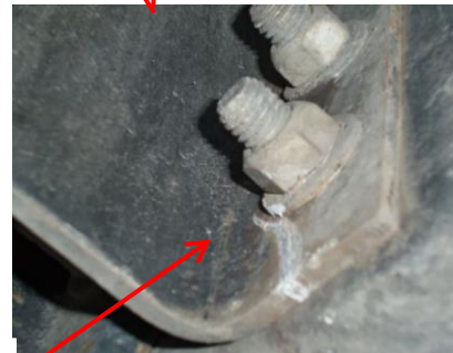
Example shown of vertical crack at lower hole. Cracks may be vertical or horizontal to one or more holes.
