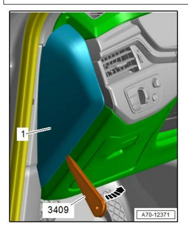
• Pry off the instrument panel side cover <1> using the -3409- in direction of <arrow>.
