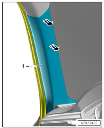
• Unclip the A-pillar gap cover <1> using the -3409- in direction of <arrow A> and disengage at the A-pillar upper trim panel in direction of <arrow B>.
