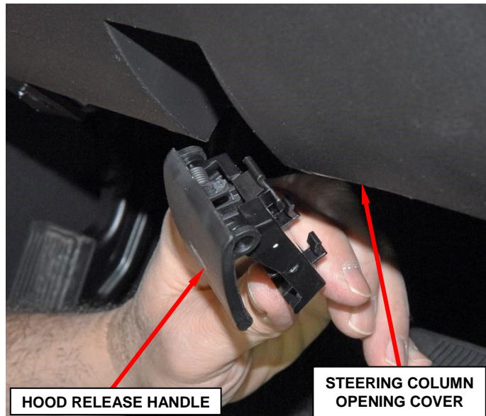
Figure 2 – Hood Release Handle
