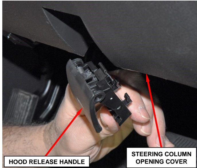
Figure 2 – Hood Release Handle
