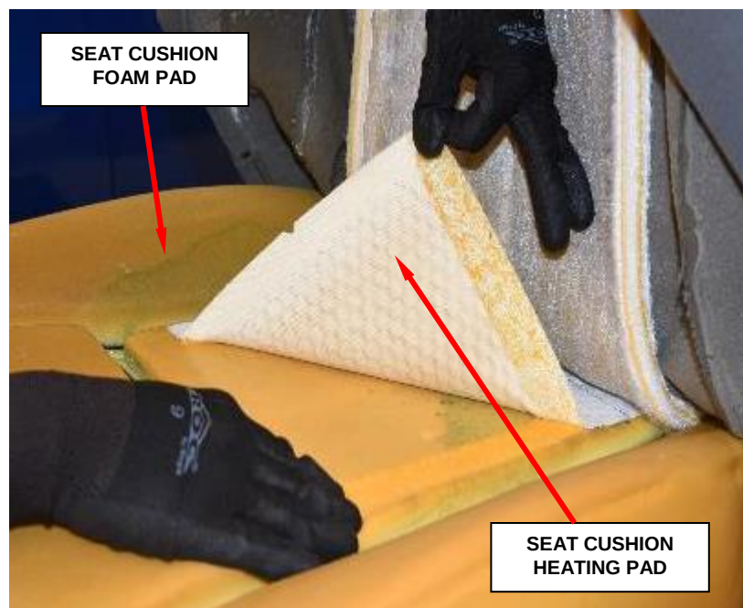
Figure 15 – Seat Cushion Heating Pad Removal
