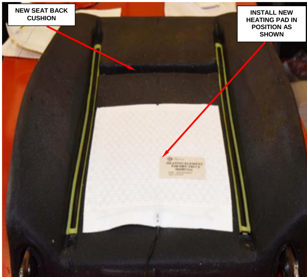
Figure 19 – Seat Back Cushion and Heating Pad Location
