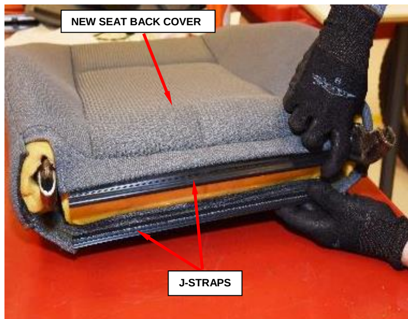
Figure 14 – Seat Back Cover J-Straps (Seat Back Removed for Photographic Purposes)
