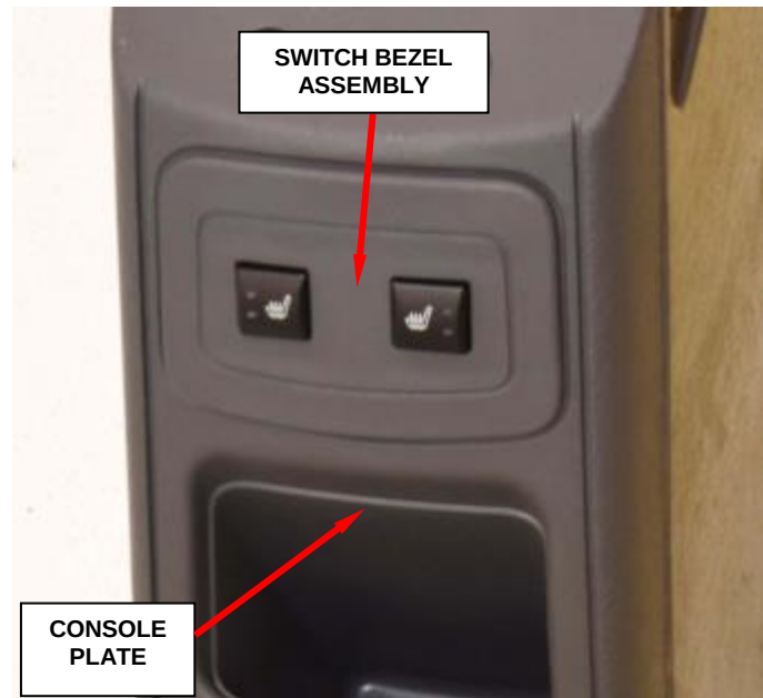
Figure 9 – Switch Bezel to Console Plate
