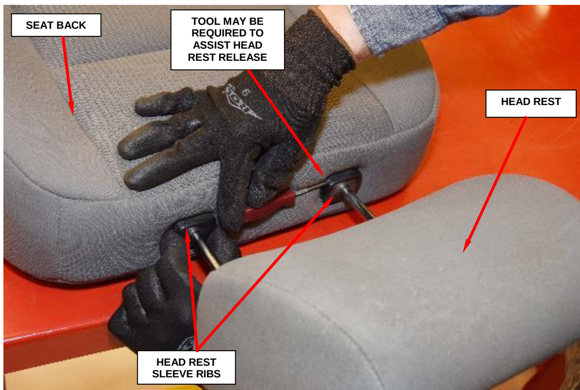
Figure 18 – Head Rest Removal
