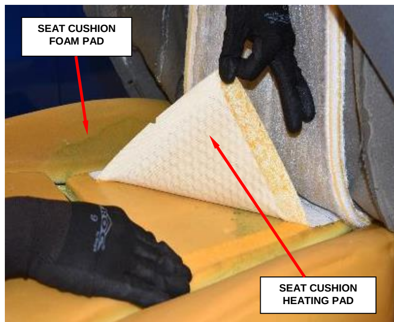
Figure 15 – Seat Cushion Heating Pad Removal
