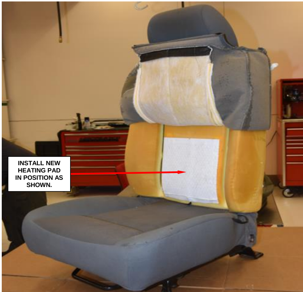
Figure 13 – Heating Pad Location
