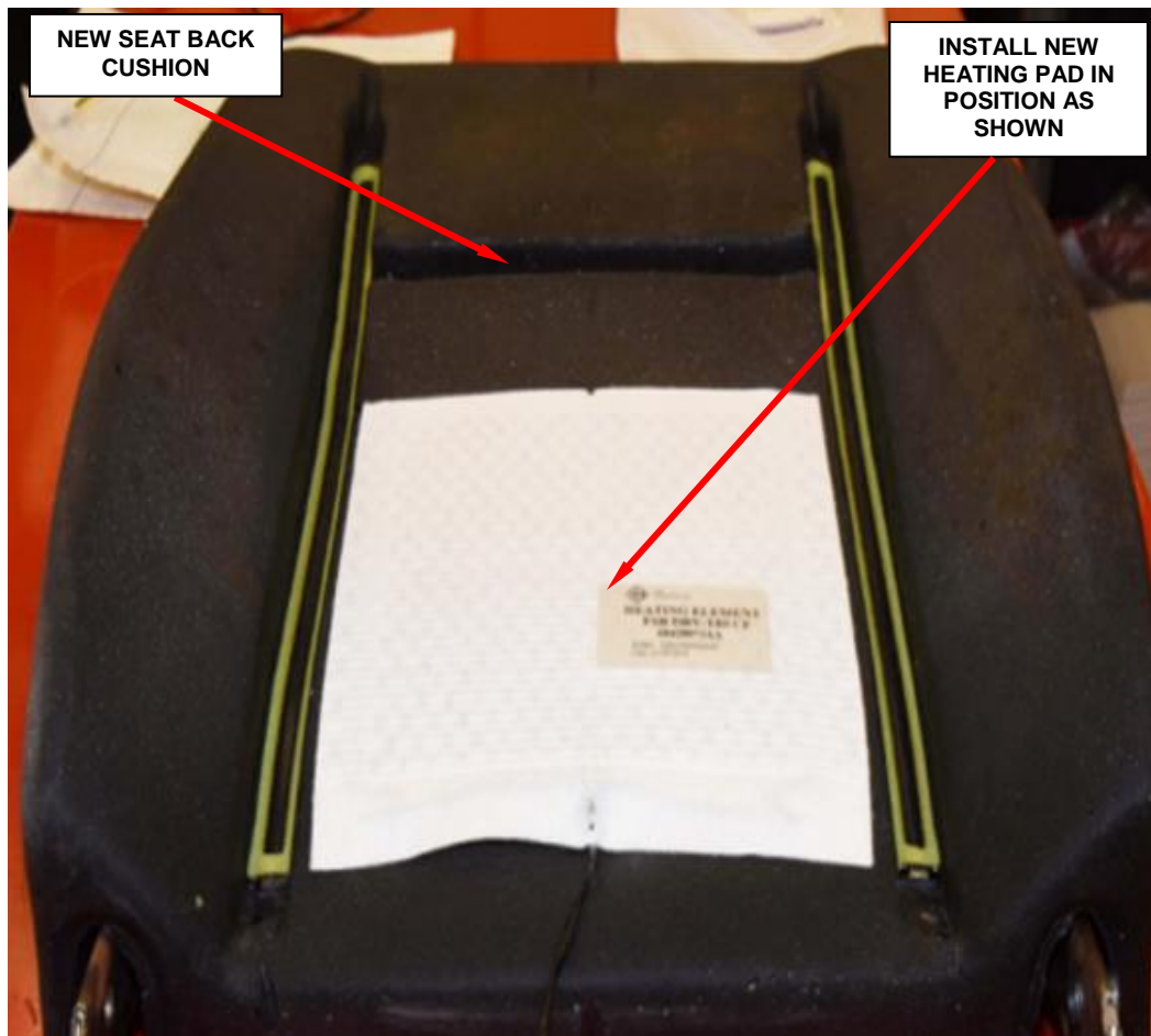
Figure 19 – Seat Back Cushion and Heating Pad Location
