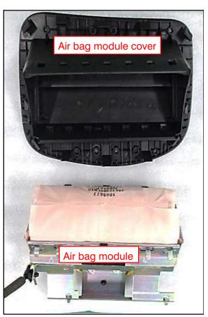
18. Continue rotating the air bag module until it fully separates from the cover.
