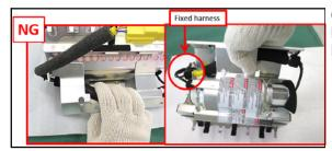
**CAUTION:** Do NOT pull on the harness or hold the harness while handling the air bag inflator module. The harness may separate or disconnect as a result.
