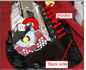
14. Rotate the air bag module toward the Back side, in the direction of the arrow (1), to clear the hooks from the holes.
