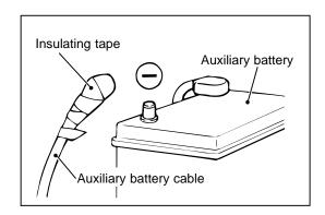
Record the radio station presets. Disconnect the negative (-) auxiliary battery cable and insulate the terminal with electrical tape.
