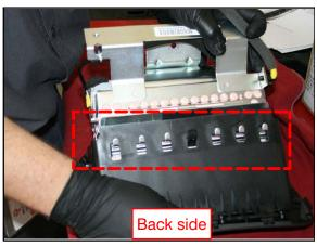
6. Confirm that the air bag module is correctly hooked into place.
