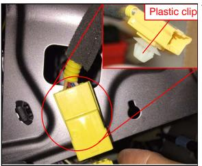
7. Gently pry the air bag module harness' plastic clip from the metal dash brace.
