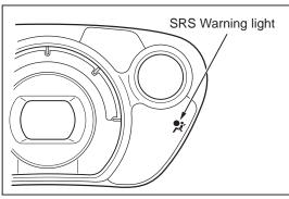
8. Turn the electric motor switch to the "ON" position. If the "SRS" warning light illuminates continuously (does not extinguish after eight seconds), troubleshoot per the applicable service manual, Group 52B — Supplemental Restraint System (SRS) > SRS Air Bag Diagnosis > SRS Warning Light Check.
