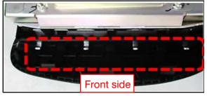
4. Confirm that the air bag module is correctly hooked into place.
