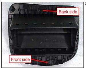
2. Identify the Front and Back sides of the air bag module cover.
