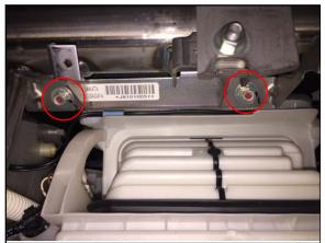
8. Unbolt the air bag module from the metal dash brace.
