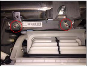
2. Bolt the air bag module to the metal dash brace to  $44\pm8$  in–lb (5.0  $\pm$  1.0 Nm).
