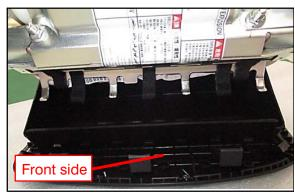
3. Align the warning label side of the air bag module toward the Front of the air bag module cover. Hook the air bag module into the appropriate air bag module cover holes.
