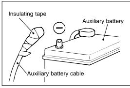
7. Remove the electrical tape and reconnect the negative (-) auxiliary battery terminal. Tighten the clamp nut to  $44\pm8$  in-lb ( $5.0\pm1.0$  Nm).
