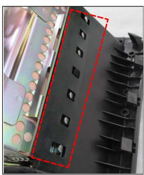
15. Verify that the (7) hooks appear retracted from the air bag module cover.
