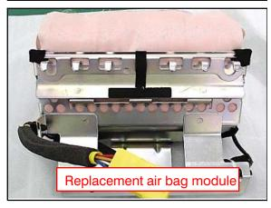
1. Verify that the replacement air bag inflator module appears intact. Light surface rust may be present on the inflator surface. This is normal and does not affect the functionality of the inflator.
