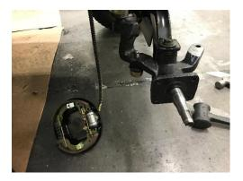
• Remove the (4) 13mm fasteners show here.
