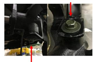
• Remove the 17mm kingpin fastener and nut.
