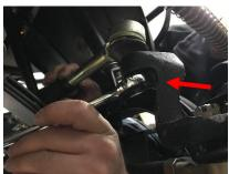
• Remove the (4) 19mm lugnuts holding the wheel onto the hub.
