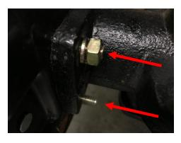
• Remove tie rod link after removing 19mm castle nut.
