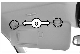
7. Using a pick tool, carefully pull open the two (2) assist handle caps. Remove the two (2) assist handle retaining screws (H) and remove the assist handle. Repeat for the remaining three (3) assist handles located on the roof trim (headliner).
