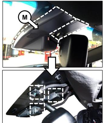
Disconnect the front roof trim connectors located at both driver and passenger Apillars.
