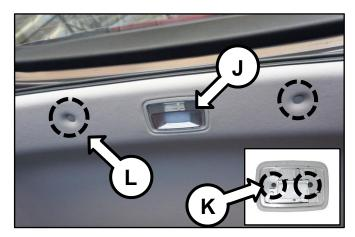
10. If equipped with center room lamp (nonpanoramic roof models), carefully remove the room lamp lens using a small flat-tip screwdriver. Remove the two (2) lamp retaining screws (J) and lower the room lamp then disconnect the room lamp connector and remove the lamp.
