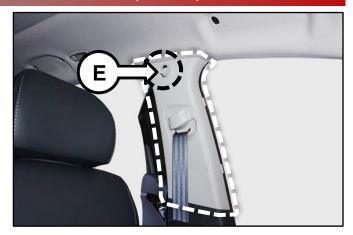
5. Using a pick tool, carefully pull open the C-pillar bolt cover and remove the rear C-pillar trim retaining bolt (F). Use a non-marring trim removal tool and remove the C-pillar trim and let hang from seat belt. Repeat for the opposite side.
