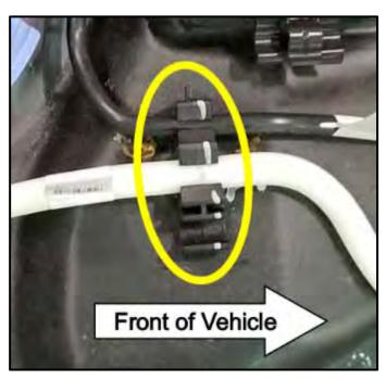
• Note the installation position of the fuel line and vent line.
