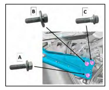
Install the following bolts in their respective locations and torque to 70 Nm + 90°.
