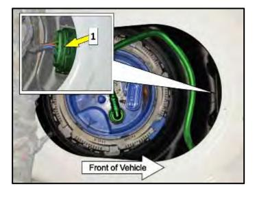
Disconnect the Fuel Pump Control Module -J538- <1>.
