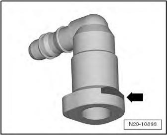
Press the release button <arrow> and remove the connector coupling from the fuel delivery unit.
