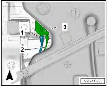
Connect the fuel line <2> and the breather line <1> on the underbody.
