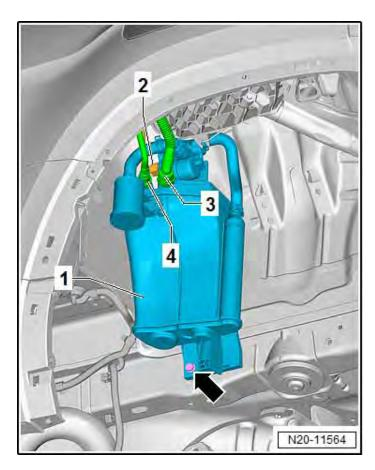
Release and remove the breather lines <3 and 4> from the charcoal canister <1>.
