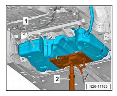
• Place the -VAS6931- <2> under the fuel tank <1> to support it as shown.
