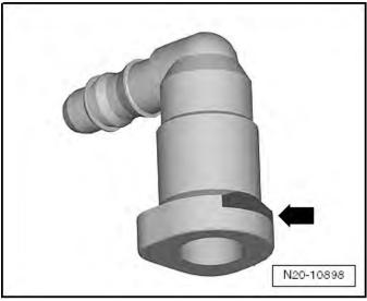
• Press the release button <arrow> and remove the connector couplings from the fuel lines.
