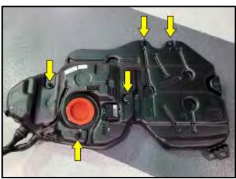
Ensure the rubber bumpers <arrows> are fully seated onto the new fuel tank.
