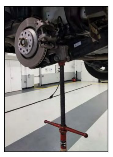
Support the wheel bearing housing with a screw jack.
