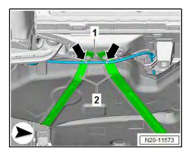
Unclip the wiring harness <1> on the mounting straps <2> <arrows>.
