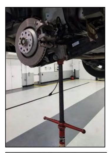
Support the wheel bearing housing with a screw jack so the trailing arm to wheel bearing housing bolt holes align.
