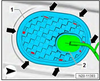
Install the sealing flange cover <1>.
