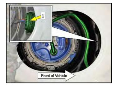
• Connect Fuel Pump Control Module -J538-<1>.
