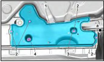
Remove the nuts <4> and bolts <2> and remove the right rear underbody trim panel <1> toward the rear <arrow a>.
