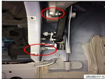
A. Visually check if all components are contacting without space in between.
