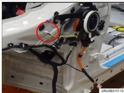
A. Ground point of charging receptacle needs to be torqued to 8 Nm thru wheel housing.
