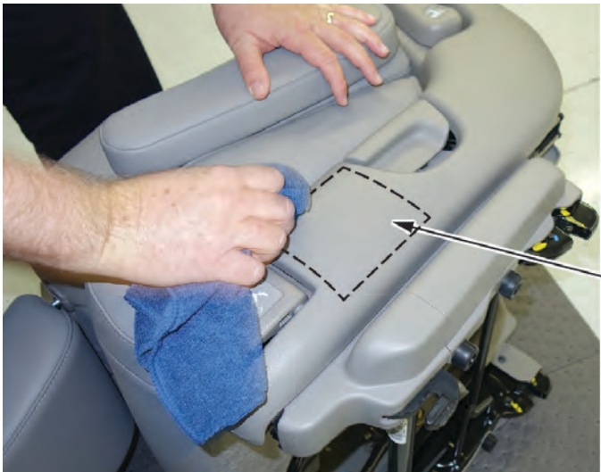
Thoroughly clean area with isopropyl alcohol.
