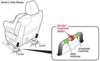
If despite the risks, a customer chooses to tip the entire second row seat forward to access the third row, they need to make sure the seat is in the standard or wide position when lowering and latching the seat.
