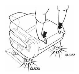
5. Raise the seat-back to an upright position, then rock the seat back and forth, trying to tilt it forward, and make sure both the inner and outer latches are locked in position.
