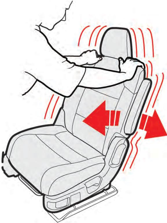
7. If the seat was installed in the wide position when the vehicle arrived (see step 1), move the seat to the wide position for the owner's convenience. Make sure both front seat hooks are fully inserted in the floor strikers and rock the seat back and forth to confirm both the inner and outer latches are securely locked into position.
