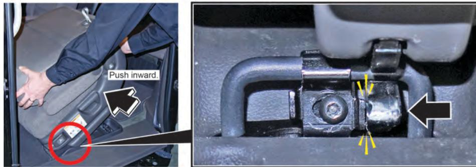
6.1.3. After confirming both front hooks are fully inserted into the front strikers, begin to lower the seat then allow it to drop and lock to the rear floor strikers.
