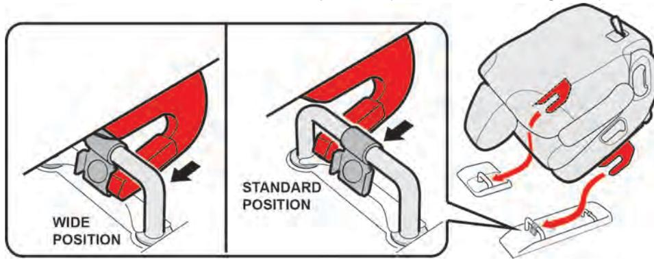
6.1.2. Next, push the seat in toward the center of the vehicle until the front outer hook contacts the countermeasure bracket as shown.
