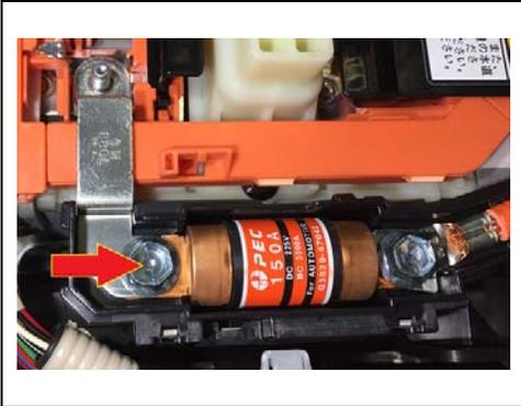
b. Remove the bolt using the insulated 8mm or 10mm magnetic extension (depending on application) and insulated ratchet from the HEV workstation.
