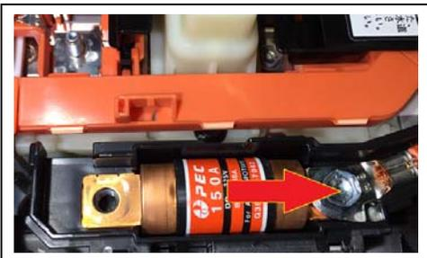
d. Remove the bolt using the insulated 8mm or 10mm magnetic extension and insulated ratchet from the HEV workstation.
