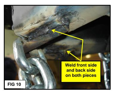
**Fig 9:** Weld both **ends** of each chain elbow to A-Frame. Weld the outside and the inside on each end of the chain elbow to A-Frame. **Fig 10:** Front and back sides of each end of the chain elbow(s) should be welded to the A Frame.
