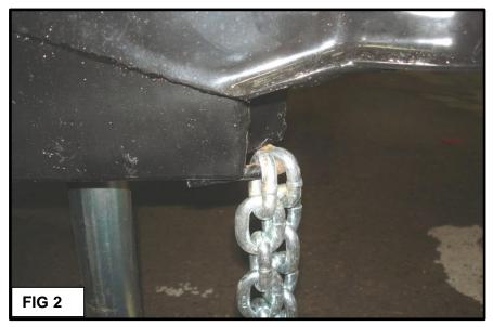
1 Fig 1: Locate the safety chains and the chain elbow(s) under the hitch coupler.
