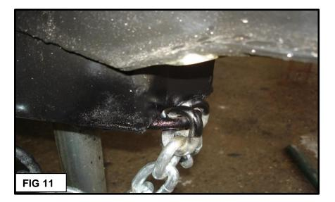
Fig 11: Once welds are cool, paint black with a good quality spray paint like Rustoleum. Chains should move freely on the chain elbow.
