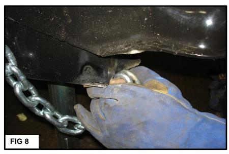
4 Fig 7: Hook the new chains on top of the A-Frame. Insert the new chain elbow(s) through the new two chains . Fig 8: Hold the chain elbow(s) up under the hitch where the old one was located. Make sure the elbow is positioned out far enough to ensure the chains can move freely on it Move the chains over to one side away from welding area.
