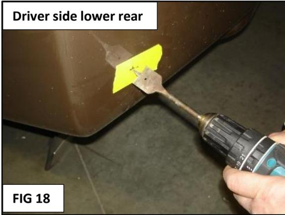
**FIG 18:** Use the drill with the 1-1/4" drill bit.
