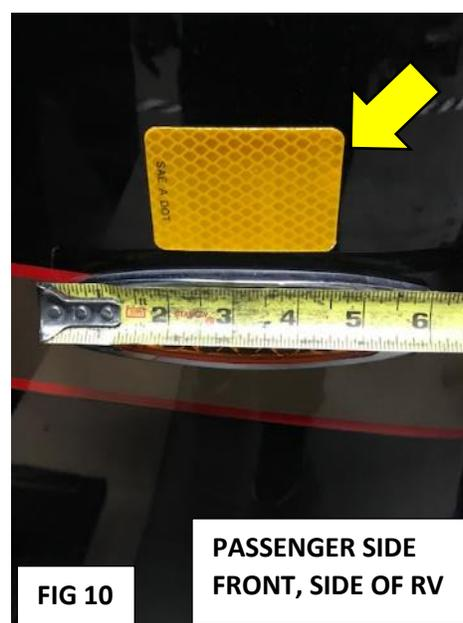
**FIG 9:** Place an amber reflector 1/4" above the front side marker light.
