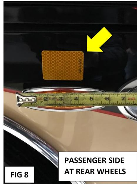
**FIG 7:** Place an amber reflector 3/8" above the intermediate marker light (located just in front of the rear dual wheels)
