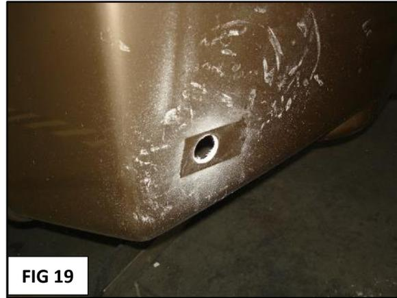
**FIG 19:** Clean off the fiberglass dust around the holes.
