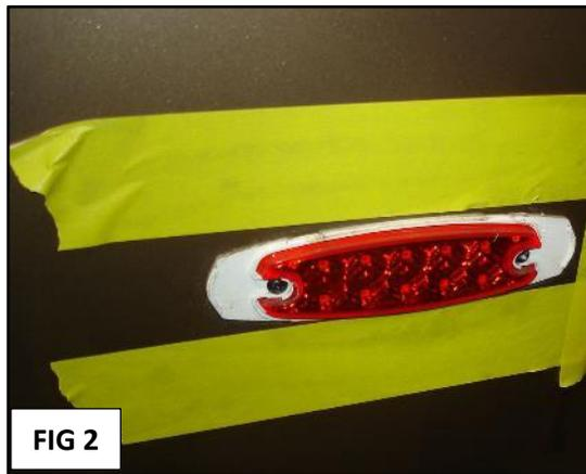
**FIG 1:** Tape around the existing marker light as a guide for placement of new light. Gently pry off the chrome bezel using the plastic putty tool and a flat screwdriver. There are four tabs under the bezel holding it to the light base.
