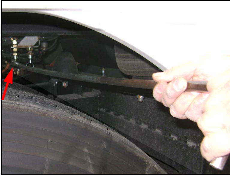
Figure 1. Reference photo of utilizing a hook rod on the tank automatic drain valve.
