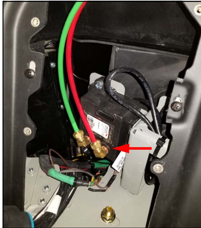
Figure 3. Dual air transducer location.
