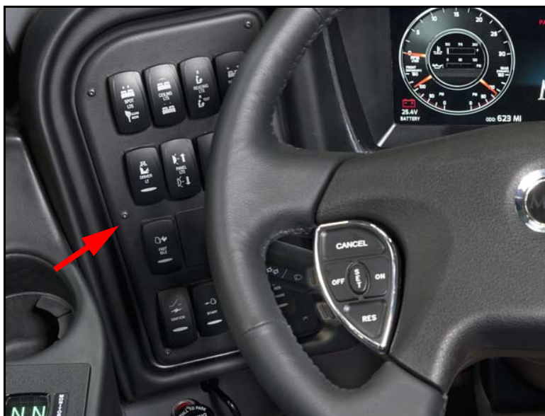
Figure 2. LH switch panel location on the instrument panel.
