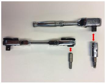
6. Use a suitable tool with T25 Torx bit to release the screws.
