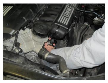
7. Reach under the intake with your left hand/arm to access the crankcase ventilation heater.
