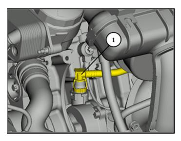
Unlock and pull off the vacuum line (1).
