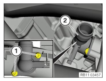
10. Install the crankcase ventilation heater (2).
