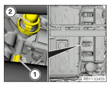
Unlock and disconnect the plug connection (1).
