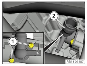
9. Install the crankcase ventilation heater (2).
