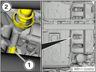
Unlock and disconnect the plug connection (1).
