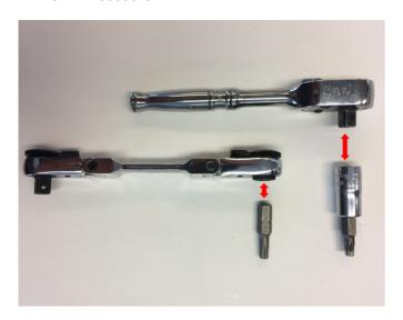
5. Use a suitable tool with T25 Torx bit to release the screws.
