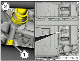
Unlock and disconnect the plug connection (1).
