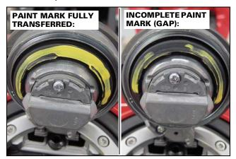
• If the paint mark was fully transferred to the seal with no gaps, the fuel cap is sealing.
