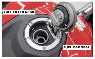
2. Apply a thin coat of bright colored waterbased craft paint to the front half of the fuel filler neck as shown.
