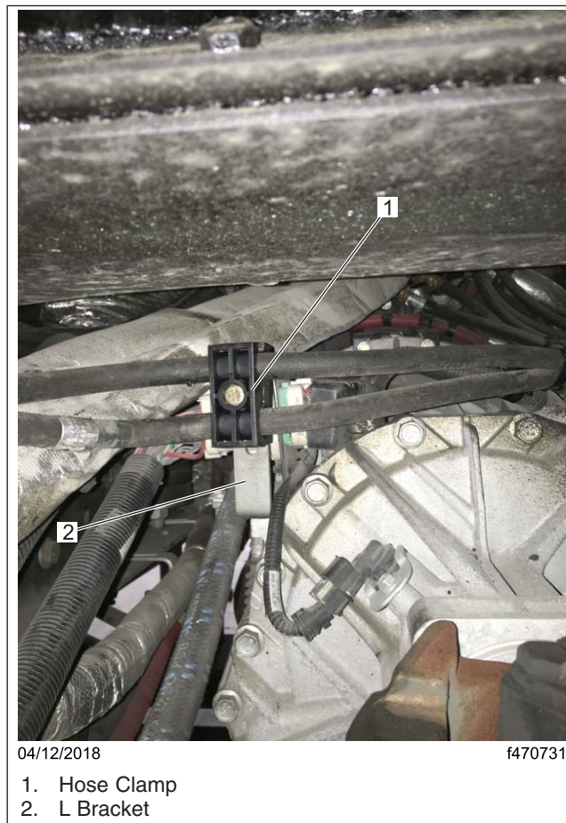
Fig. 4, Final Hose Clamp Assembly
