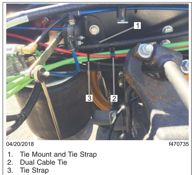
Fig. 14, Air Line Routing, Single Height Control Valve
