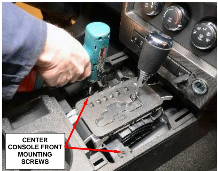
**Figure 11 – Center Console Front Mounting Screws**
