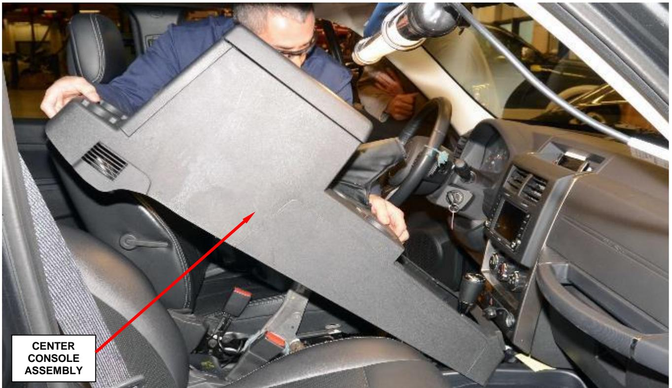
**Figure 14 – Center Console Assembly**
