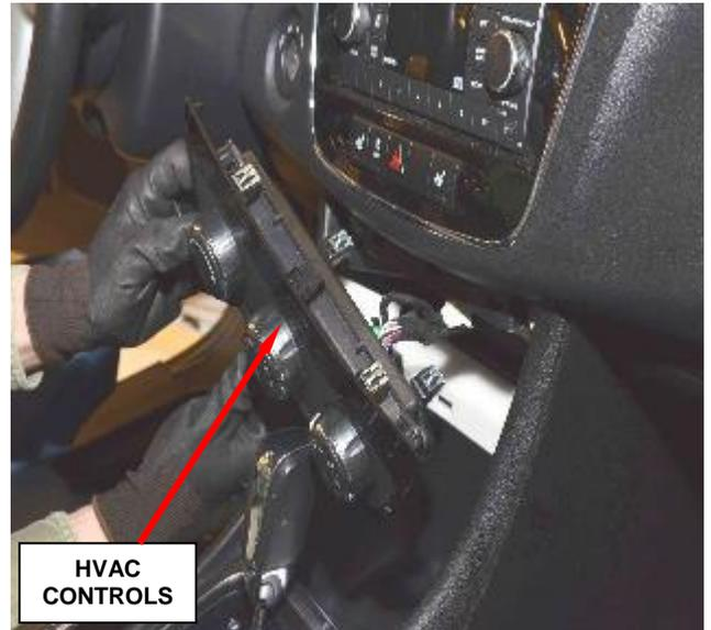
**Figure 1 - HVAC Controls**
