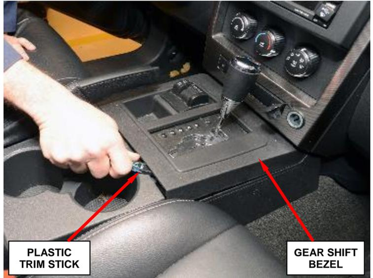
**Figure 10 – Gear Shift Bezel**
