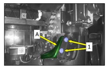
• If equipped, install the Headlamp Range Control Module <1> and connect connector <2>.
