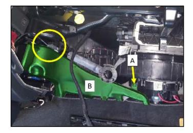
• Remove the screw clips <A> and remove the insulation mat <B>.
