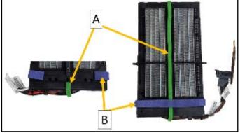
Remove the Auxiliary Heater Heating Element -Z35- <A> from the A/C unit in direction of <arrows>.
