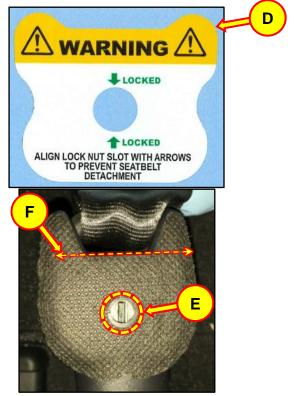
4. Firmly press down on the label to ensure it adheres to the surface of the linkage element.
