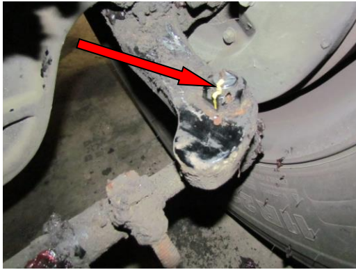
Paint Mark to Identify Nut Rotation
