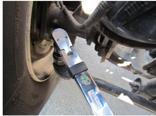
Check Nut Torque – Do Not Exceed 170 ft. lbs.
