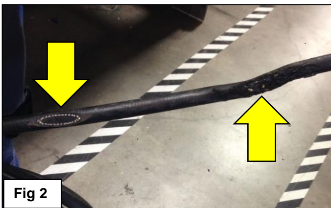
FIG 2: Damage to the LP hose: Left Arrow: rubbing from the driveshaft, Right Arrow: burnt/melted from the exhaust.
