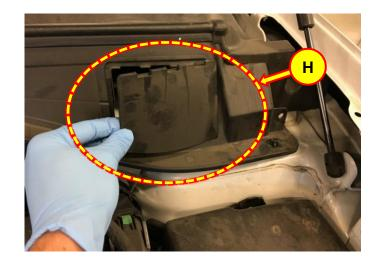
8. Remove the left hand side mounting retainer (J) and pull the cowl top cover slightly to the side to allow access to the strut mounting nuts.
