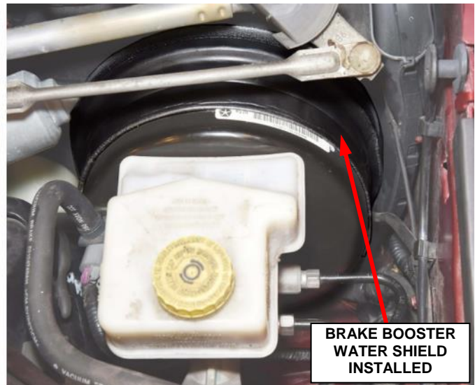
WATER SHIELD INSTALLED
