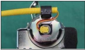
22. Clip the wiring harness to the mounting bracket as shown.
