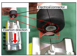
Begin insertion of the replacement inflator into the housing as shown, with the electrical connector side going in first.
