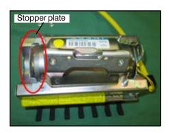
4. Remove and keep the stopper plate for reuse.
