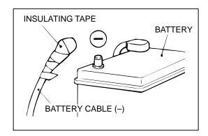
1. Record the radio station presets. Disconnect the negative (—) battery terminal and insulate the terminal with electrical tape.
