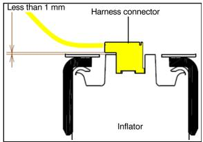
21. Ensure the harness connector is completely inserted into the electrical connector socket by gently pulling on the harness connector.
