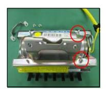
5. Loosen, but do not remove, the circled nuts.
