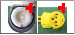
19. Match the wiring harness connector's plug with the shape in the electrical connector socket.
