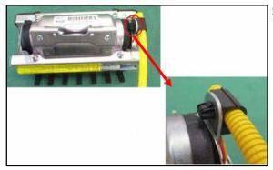
23. Confirm that the wiring harness clip has been fully inserted.
