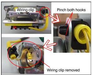
2. Use pliers to pinch the hooks and remove the wiring clip from the bracket.
