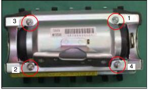
18. In the illustrated order, torque all (4) nuts to 34.5  $\pm$  3.5 in—lb (3.9  $\pm$  0.4 Nm).
