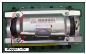
15. Install and lightly tighten the (2) nuts holding the stopper plate.
