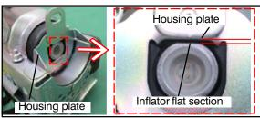
12. Ensure that the inflator makes complete contact with the housing plate. If needed, rotate the inflator so that the inflator's flat section is parallel with the housing plate.
