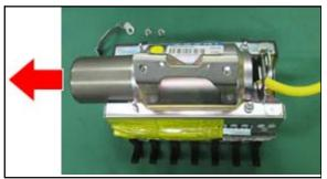
7. Gently push the inflator with your finger in the indicated direction while gently pulling (straightening) the wire to remove the inflator.
