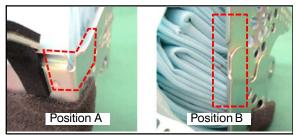
a. Note the taping area for Position A and Position B.
