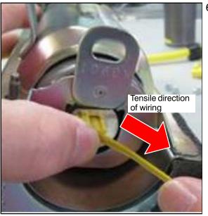
6. Gently pull and straighten the wires so it is in line with the inflator. This will prevent the wire from contacting the edges of the inflator housing during removal.
