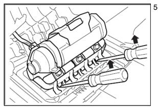
The front passenger side air bag module is secured to the instrument panel in a flexible plastic enclosure. Insert a flat head screwdriver and disengage the mounting hooks to dislodge the module from the enclosure.
