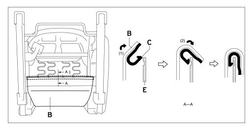
13. Confirm that the cushion pad is not exposed. Correct if necessary.
