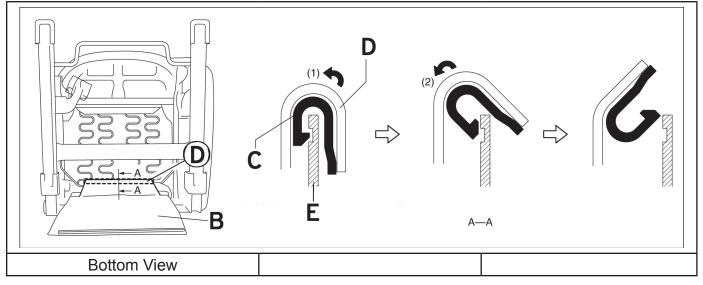
Move the hook (C) in the order of arrows (1) and (2). Set the inner trim (D) away from the front seat cushion frame (E). If it is difficult to remove the hook of the inner trim because of its tension, roll and grab the outer trim (B) and gently pull down to reduce the tension of the inner trim.
