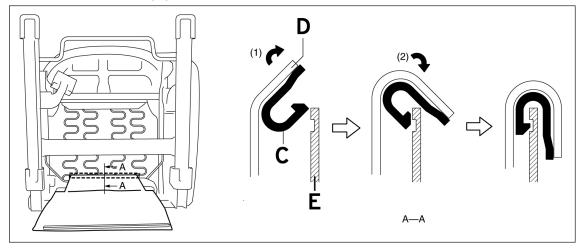
c. Pull the outer trim (B) in the direction of the arrow shown. Remove the wrinkles on the front seat cushion trim.
