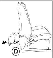
b. Move the hook (C) in the order of arrows (1) and (2) shown. Install the inner trim (D) to the front seat cushion frame (E).
