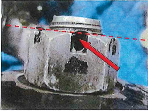
Good Cotter Pin Hole Position
