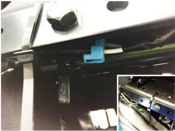
Example of left hand, normally-closed buckle
