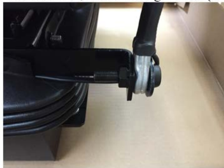
Shifted tether bar N/C buckle
