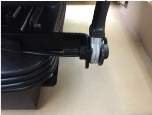
Shifted tether bar N/C buckle
