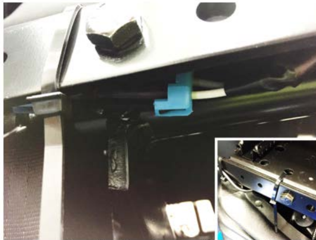
Example of left hand, normally-closed buckle
