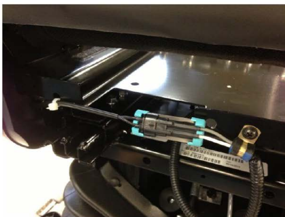
Buckle on LH side of seat
