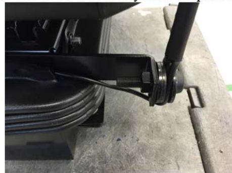
Shifted tether bar N/O buckle
