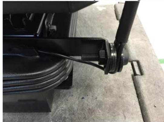
Shifted tether bar N/O buckle
