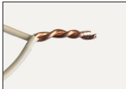
Figure 3 Properly joined solid copper wire
