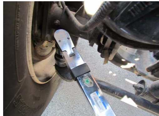
Check Nut Torque – Do Not Exceed 230 Nm (170 ft-lb)
