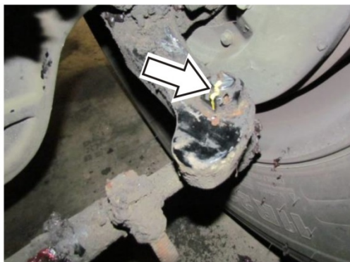
Paint Mark to Identify Nut Rotation
