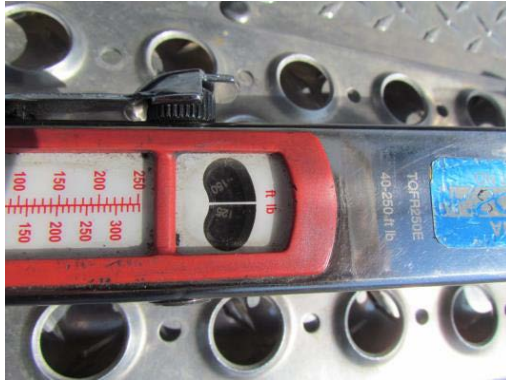
Re-torque to 176 Nm (130 ft-lb)
