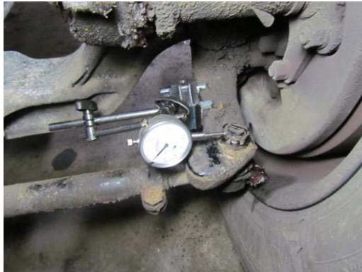
Dial Indicator Mounting Position
