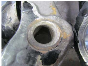
Tie Rod Arm Taper Bore
