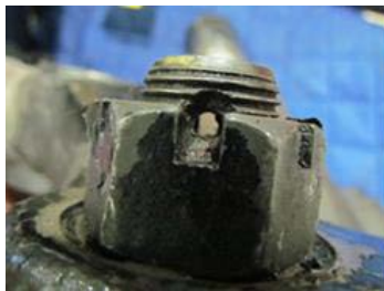
Cotter Pin Hole Position
