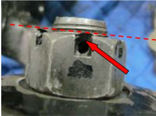
Good Cotter Pin Hole Position
