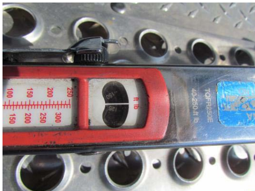
Re-torque to 176 Nm (130 ft-lb)
