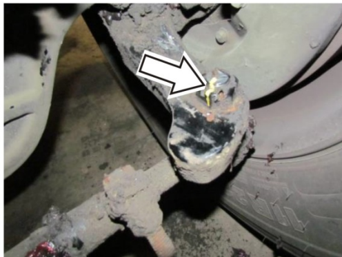
Paint Mark to Identify Nut Rotation
