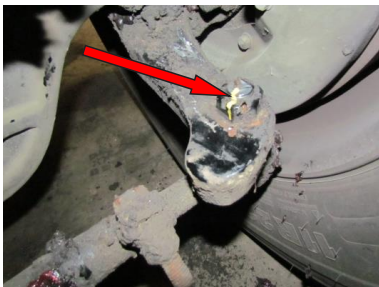
Paint Mark to Identify Nut Rotation
