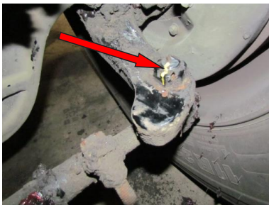
Paint Mark to Identify Nut Rotation
