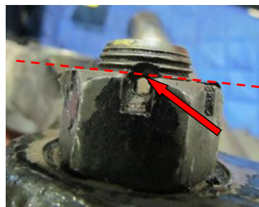
Cotter Pin Hole at Maximum Height
