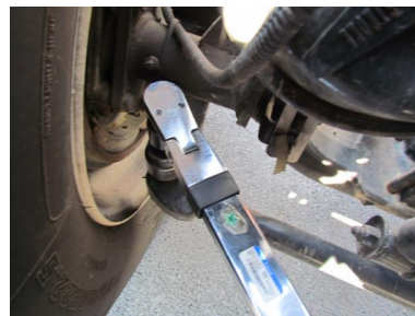
Check Nut Torque – Do Not Exceed 170 ft. lbs.
