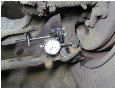
Dial Indicator Mounting Position
