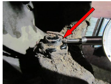
Dial Indicator Tip Must be Placed on The Stud
