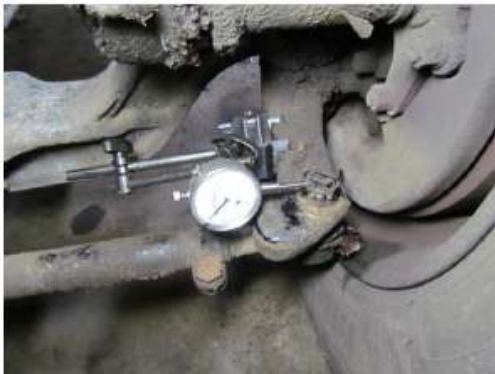
Dial Indicator Mounting Position
