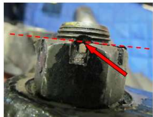
Cotter Pin Hole at Maximum Height
