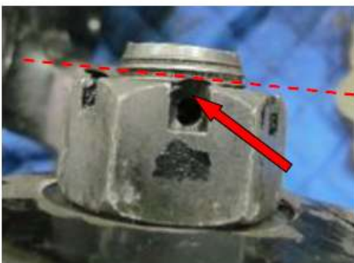
Good Cotter Pin Hole Position
