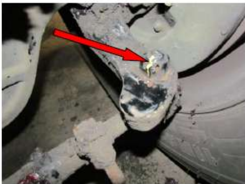
Paint Mark to Identify Nut Rotation
