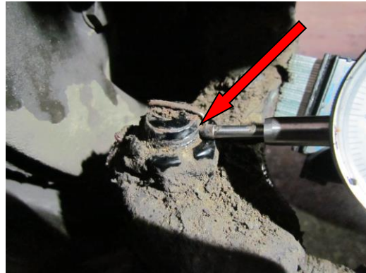
Dial Indicator Tip Must be Placed on The Stud
