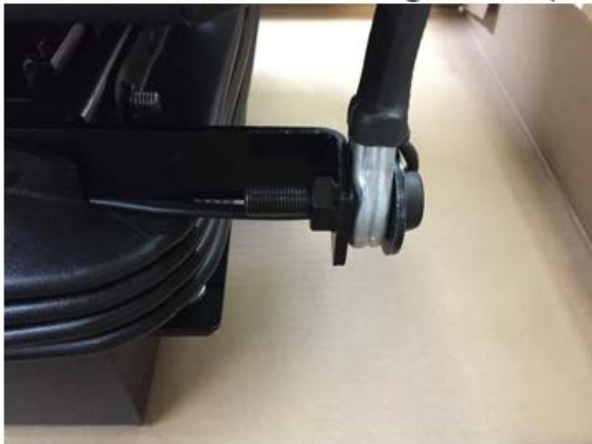
Shifted tether bar N/C buckle
