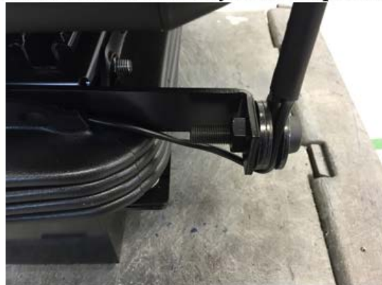
Shifted tether bar N/O buckle
