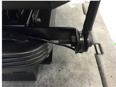
Shifted tether bar N/O buckle
