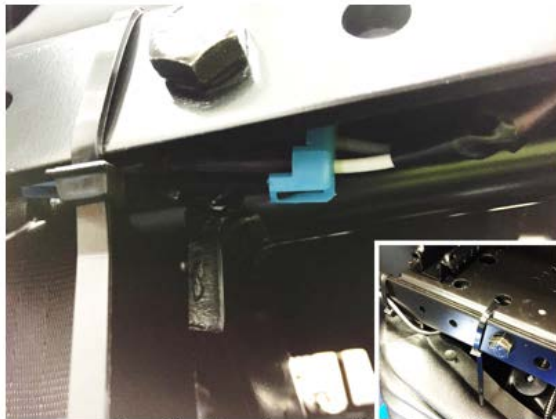
Example of left hand, normally-closed buckle
