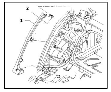
Secure harness with a 110 mm section of felt tape <1> and cable tie <2>.
