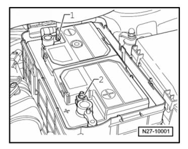
Ignition must be ON when connecting battery. If pyrotechnic components (e.g. airbag, belt tensioner) are not repaired correctly, they may deploy unintentionally after connecting battery. There must not be anyone inside the vehicle when connecting the battery.
