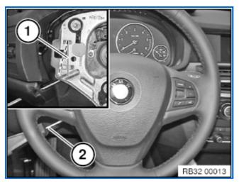
Insert Torx screwdriver T25 (2) at an angle into concealed opening on reverse side of steering wheel until a spring resistance is felt (approx. 1.5 cm).
