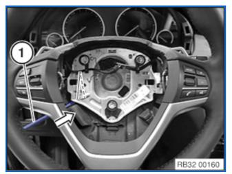
Insert Torx screwdriver T30 (1) at an angle into concealed opening on reverse side of steering wheel until a spring resistance is felt (approx. 2 cm).
