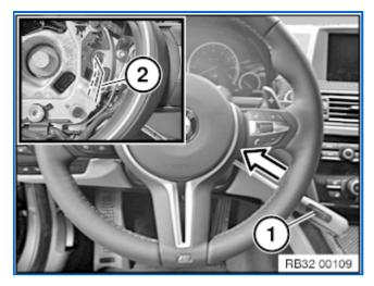
Insert Torx screwdriver T27 (1) straight into concealed opening until a spring resistance can be felt.
