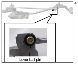
4. Use a rag to clean dirt and grease off of the lever ball pin and rubber seal.
