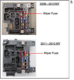
Using the Fuse Remover, locate and remove the green (30 A) Wiper Fuse.
