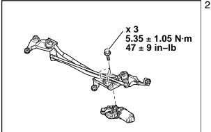
21. Install the wiper motor to the wiper link assembly as illustrated, and tighten the 3 bolts to  $47 \pm 9$  in–lb (5.35  $\pm$  1.05 Nm).
