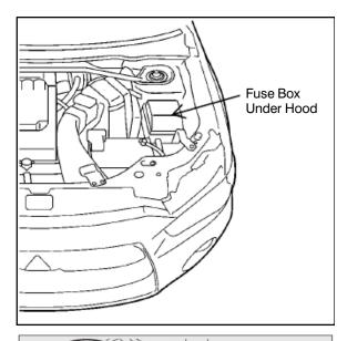
1. Obtain the Fuse Remover from the engine compartment fuse box.
