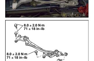
Torque bolts to 71  $\pm$  18 in–lb (8.0  $\pm$  2.0 Nm).
