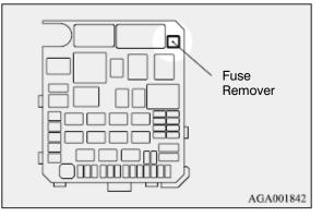
c. Remove the Fuse Remover.
