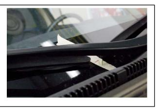
7. Remove the wiper arm blade assembly.
