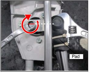
10. Make sure that the wiper motor shaft mark and the link plate center line are lined up. Use an adjustable wrench to hold the link plate in position, to prevent link plate rotation. Tighten the nut to 12.5 ft-lb  $\pm$  1 ft-lb (17.2  $\pm$  1.0 Nm).
