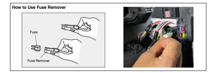
**WARNING** A Fuse Remover MUST be used to remove fuses. Use of other tools such as pliers can potentially result in thermal incidents.
