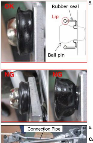
5. Verify that the rubber seal is not damaged. If rubber seal is damaged, replace it with a new rubber seal (part # 8251A098).
