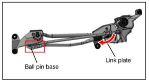
13. Turn the link plate slowly in the direction shown by the red arrow, so that the ball pin's base is visible (for easier installation).
