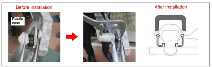
**CAUTION** The rubber seal must be properly seated. Confirm good condition of the rubber seal.
