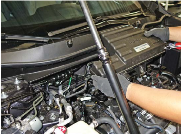
INTAKE AIR RESONATOR 2 BOLTS 12 N·m (9 lb-in)
