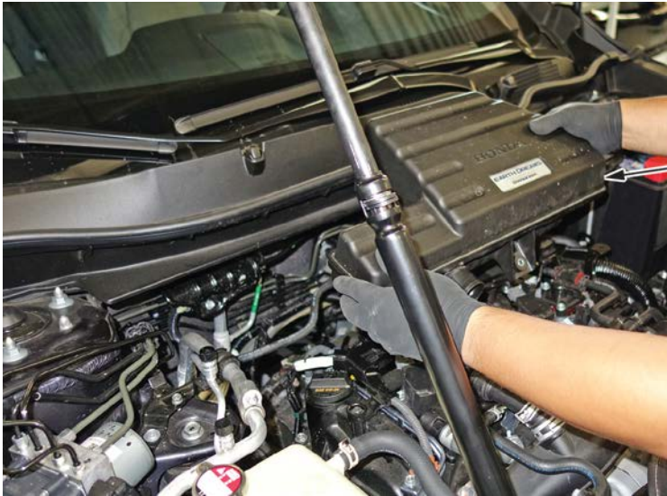
INTAKE AIR RESONATOR 2 BOLTS 12 N·m (9 lb-in)
