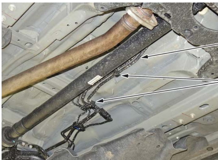
FUEL FEED PIPE Replace.
