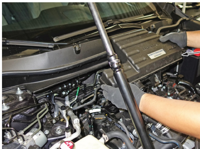
INTAKE AIR RESONATOR 2 BOLTS 12 N·m (9 lb-in)
